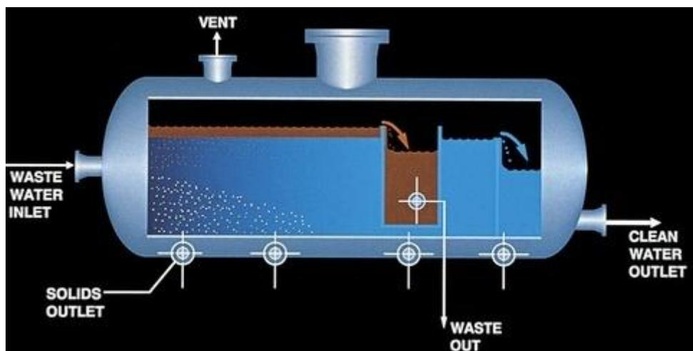
Oil/Water Separator using gravity
